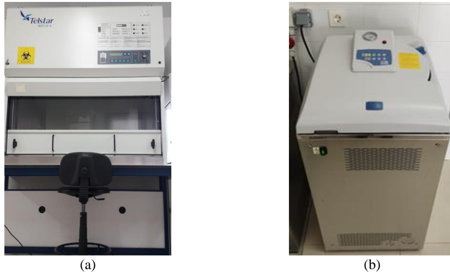
Figure 3.1. (a) Laminar flow cabinet and (b) autoclave used in this work and available at the laboratory of Solar Treatment of Water (CIEMAT-PSA).
